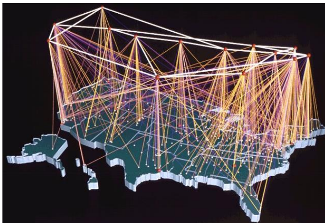
The connected dots suspended above the map represent the commercial backbone of the Internet in the USA. The vertical lines show how the various Service Providers etc. connect onto this backbone.
